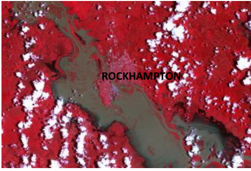
NASA IMAGE 2011 FITZROY FLOOD:-Major Fitzroy Floods:1918 (10.1m), 1954 (9.4), 1991 (9.3), 2011 (9.2m). Possible Maximum Flood (12.0m) Proposed Depot Hill Flood Levee (9.7m). Climate change prediction (10.6m) 3 Flood Study Report Fitzroy River Flood Study RRC, July 2011
